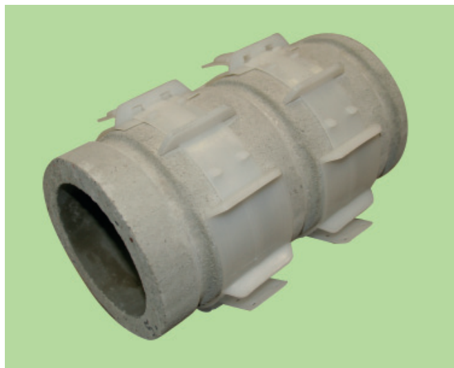
Wall sleeve with 15 mm spaces to center in core-drilled hole for the casting process
